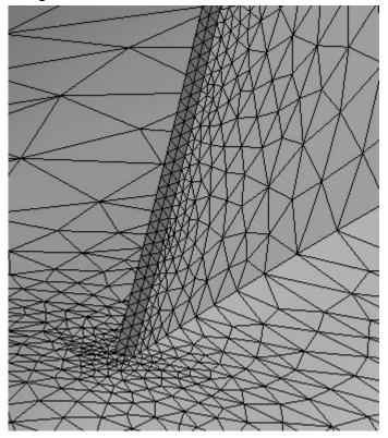
Notice how the element size is relatively uniform on the faces that were selected for the first sizing control.
