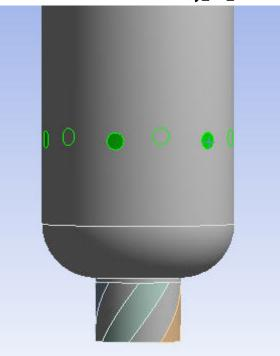
4. To create a Named Selection for the outlet, select the rectangular face with the highest Z-coordinate. Name this Named Selection **outlet**.
