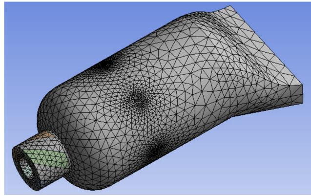
Activate a section plane to view a section cut through the model. Select Show Whole Elements
