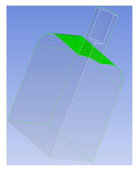
When the image above was captured, the **Draw Face Mode** option was set to **Auto Face Draw** (the default). The **Draw Face Mode** option determines whether face culling is turned on or off:
