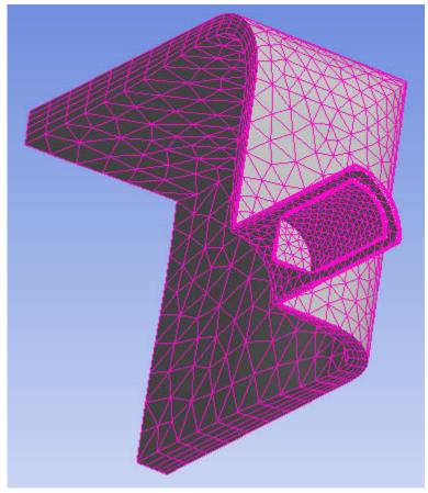
Because the **Fluent** solver was used, the meshing process used the **Layer Compression** method for **Collision Avoidance** by default.
