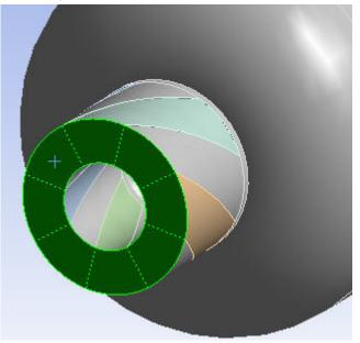
3. To create a Named Selection for the secondary air inlet, select the six small circular faces on the main body of the combustor, as shown below. These introduce extra air to aid combustion. Name this Named Selection **secondary\_air\_inlet**.
