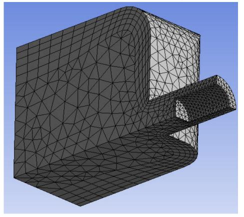
The inflation layers look different in this mesh because the **CFX** solver uses the **Stair Stepping** method of **Collision Avoidance** by default.
