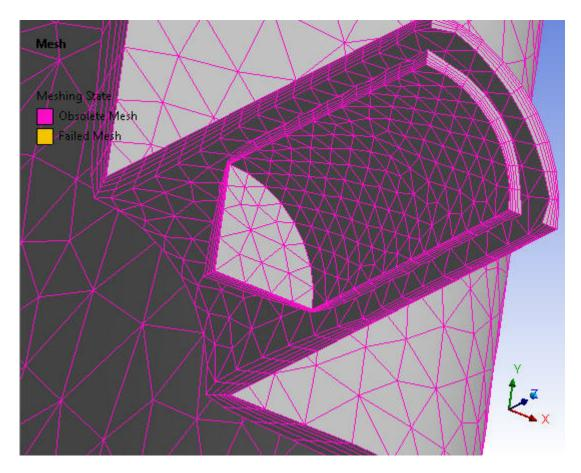
Notice the heights of the inflation layers, which are determined by the setting of the **Inflation Option** control. The **Smooth Transition** option, which was used here, uses the local tetrahedral element size to compute each local initial height and total height so that the rate of volume change is smooth.
