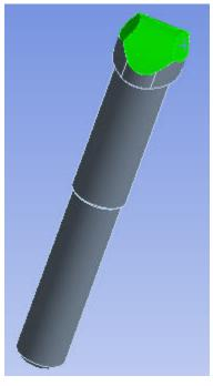
e. Right-click in the **Geometry** window and select **Insert > Virtual Cell**.
