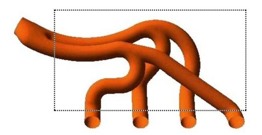
The geometry of the region of interest is then defined. If the geometry already exists in CAD, it can be imported directly. The mesh is then created. After importing the mesh into the preprocessor, other elements of the simulation including the boundary conditions (inlets, outlets, and so on) and fluid properties are defined.
