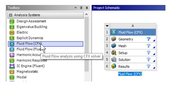
The fluid-analysis system in the **Project Schematic** shows the steps in performing a fluid analysis:
