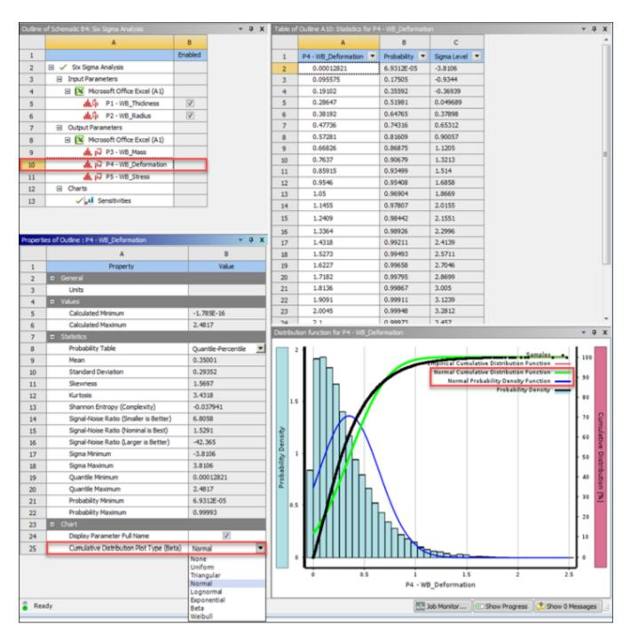
By default, **Cumulative Distribution Plot Type (Beta)** is set to **Normal**. This means that in the chart for the output parameter, the solid blue and green curves are the cumulative distribution function and probability density function based on the normal distribution.
