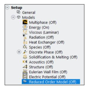
5. In the **Reduced Order Model** window that opens, select the **Enable Reduced Order Model** check box to expand the window so that you can set up the ROM.
