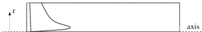
Figure 1.5: Typical Radial Distribution of Circumferential Velocity in a Free Vortex
