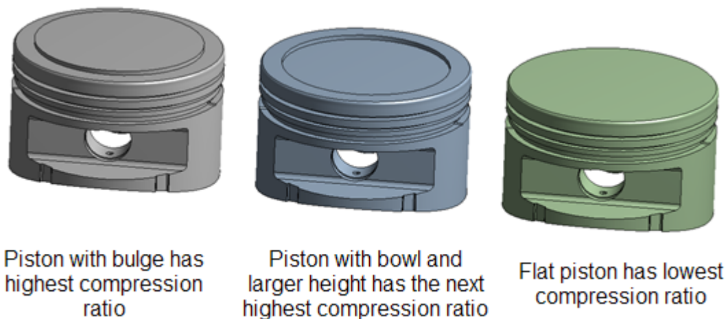
Figure 1.3: Different Piston Shapes Used to Achieve Desired Compression Ratio for an Engine
