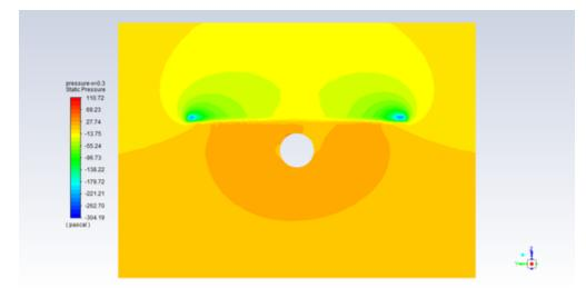
Figure 31.35: Pressure Distribution with Collective and Cyclic Trimming;X=0.3 Cutting Plane
