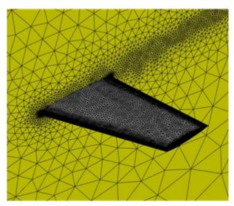
Figure 34.2: ONERA M6 wing – Mesh Detail: Leading Edge at the Wing Root (Left) and Wing Tip (Right)
