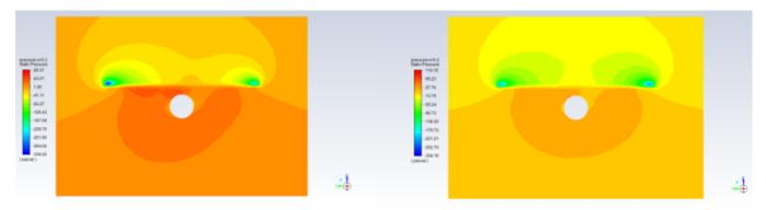
Figure 31.17: Static Pressure at the Y=0 Cutting Plane, Seen from the Side
