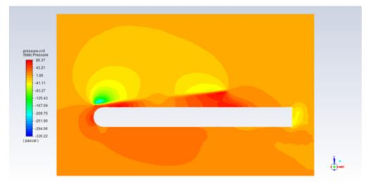
Figure 31.31: Pressure Distribution with Fixed Blade Pitch; Y=0 Cutting Plane
