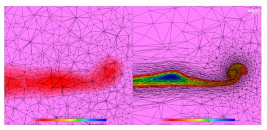
Figure 34.17: Velocity Vectors at X = 1.2m Plane, Wing Tip Vortex - Original Solution (Left) and  $2^{nd}$  Adapted Solution (Right)
