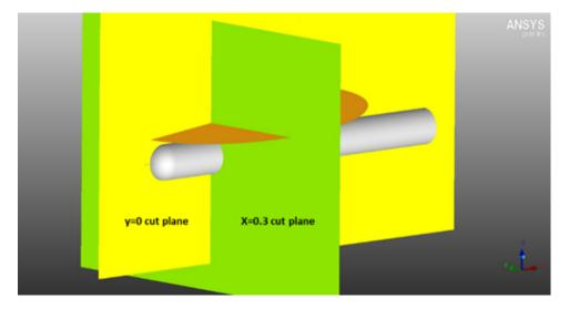
Figure 31.14: Locations of the Cutting Planes Across the Fuselage
