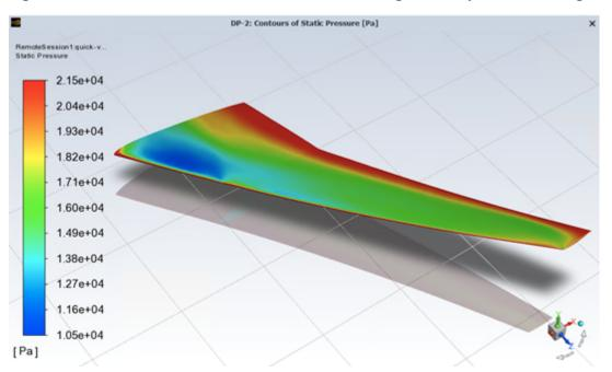
Figure 33.61: Wall Static Pressure Contour of the Wing\_01 Component of Design Point 2
