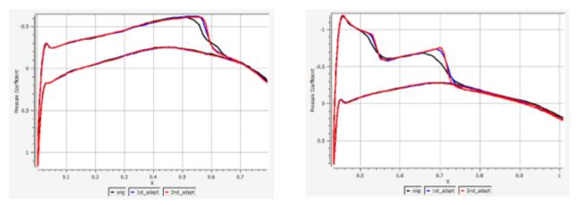
As seen from the above figures, mesh adaptation further refines the mesh at the location of the lambda shock as well as the wake produced by the wing. This extra refinement allows the airflow solver to capture the abrupt pressure drop across the lambda shock (see 2D plot figures). Other
