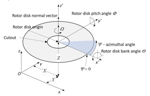
Figure 31.1: Rotor Disks Schematic
