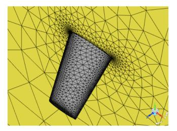
Figure 33.3: View of the Surface Mesh around the ONERA M6 Wing
