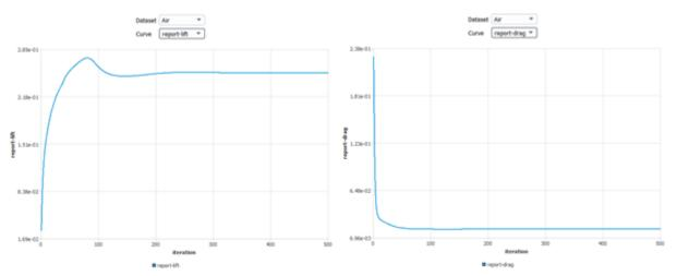
Figure 34.5: Convergence of Lift and Drag Coefficients
