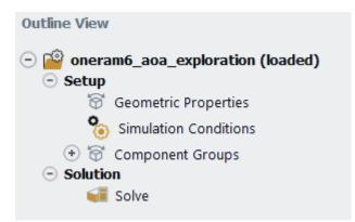
While importing, Fluent Aero will search for and find the **pressure-far-field** zone that defines the external boundary of the domain. If present, this will cause Fluent Aero to determine that this case is using a **Freestream** domain type, and the following message will be reported in the console.
