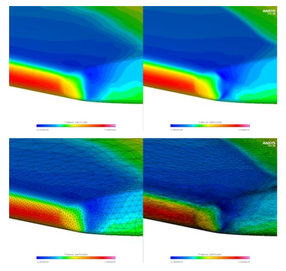
This figure shows how mesh adaptation improved the mesh refinement of the curvature of the leading edge and wing tip. As a result, a more continuous distribution of pressure coefficient along these high velocity gradient locations can be achieved.
