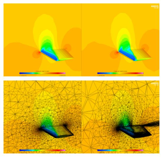
Figure 34.12: 2D Surface Pressure Coefficient Distributions Along the Wing at Z = 0 m (Left) and Z = 0.75 m (Right)
