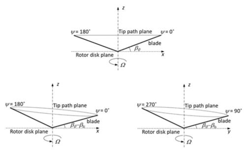
The change in the angle of attack due to flapping is computed, however the relatively small flapping velocity component  $\partial \beta / \partial t$  that should be added to the velocity component normal to the blade path is neglected. Furthermore, due to its relatively small effect, the lead-lag motion of the blade is also neglected.
