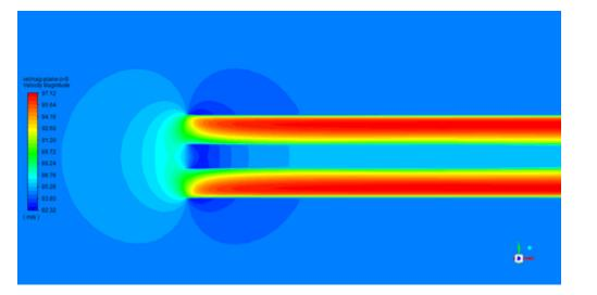
Figure 31.50: Velocity Magnitude Distribution Around the Actuator Disk; Z = 0 Cutting Plane
