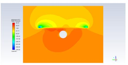
Figure 31.32: Pressure Distribution with Fixed Blade Pitch; X=0.3 Cutting Plane
