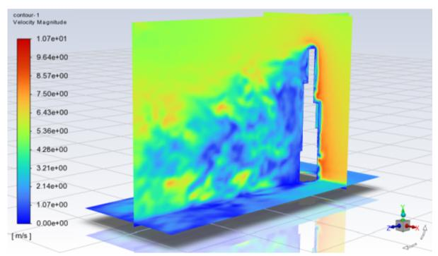
Figure 27.34: Contours of Velocity Magnitude on the YZ, ZX, and XY Planes
