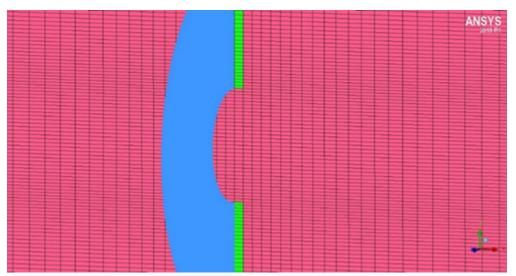
Finally, the grid in the downstream of the rotor should have sufficient clustering to capture the complex effects of the momentum change imparted by the VBM and the interaction of the wake of the rotor with other rotors (for example, main and tail rotors of a helicopter) or with other components of the aircraft/rotorcraft. Since the load distribution of a rotor is generally non-uniform, secondary vortices are likely to appear and should be captured in as much detail as possible.
