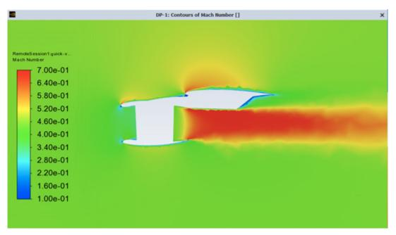
Figure 33.63: Mach Number Cutting Plane Contour of Design Point 1
