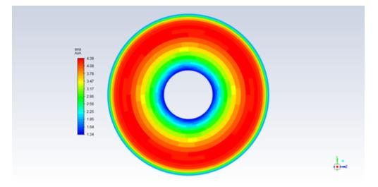
Figure 31.57: Blade Pitch Angle Distribution on the Actuator Disk with Collective Trimming
