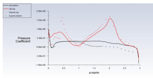
Figure 31.39: Pressure Coefficient Distribution Along the Port and Starboard Sides of the Fuselage Obtained with Collective and Cyclic Trimming
