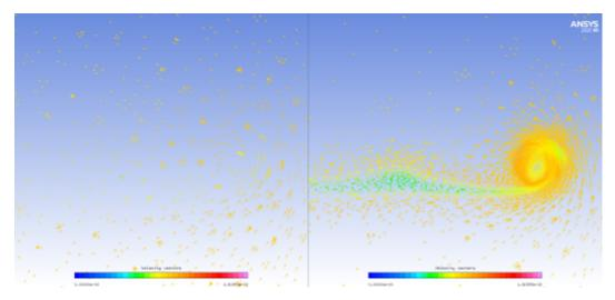
The above figures show the level of mesh refinement that was added during mesh adaptation cycles in order to precisely capture the wake and the wing tip vortex produced by the wing. These phenomena are important to capture especially for high lift configurations or aircraft components that are located in the wake of upstream surfaces.
