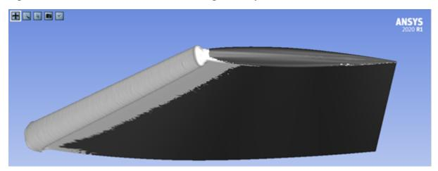
Figure 32.1: Multishot Automatic Remeshing Ice Shape
