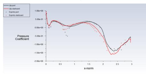
Some improvements in the agreement between the experimental and numerical results with collective and cyclic trimming are seen at the top of the fuselage. The numerical results on the port and starboard side have also improved considerably.
