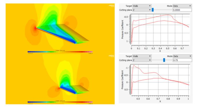
Figure 34.7: Pressure Coefficient Contours and 2D Plots at Z = 0 m Plane (Top) and Z = 0.75 m Plane (Bottom)
