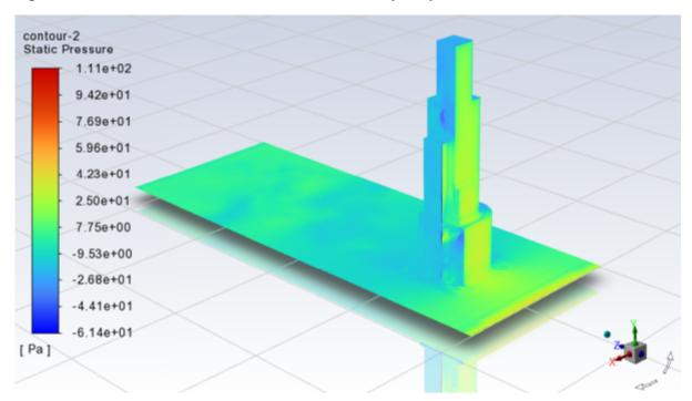
Figure 27.35: Contours of Static Pressure on the Skyscraper Walls
