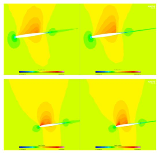
Comparison of Mach number contours show that mesh adaptation provides a clear representation of the airflow acceleration around the wing and the sudden deceleration across the shocks. Numerical noise and dissipation have been extensively reduced and the wake has been neatly captured.
