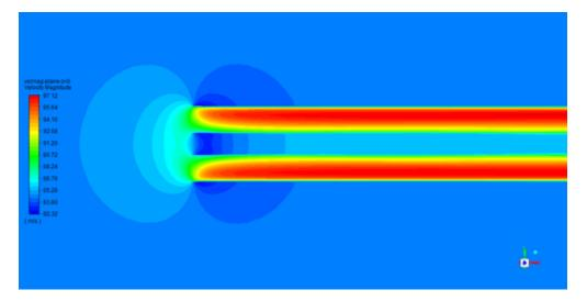
Figure 31.55: Velocity Magnitude Distribution Around the Actuator Disk with Collective Trimming; Z = 0 Cutting Plane
