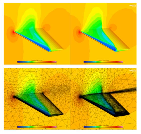
Figure 34.11: Pressure Coefficient Contours and Surface Mesh Along the Wing and Z = 0.75 m Plane - Original Solution (Left) and 2<sup>nd</sup> Adapted Solution (Right)
