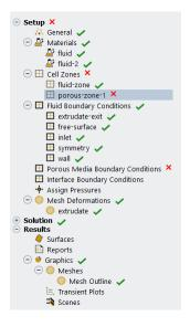
In the Outline View, the simulation can be defined by adding objects to the **Setup** section of the tree, solution-specific options are accessible from the **Solution** section, while the data from a simulation can be analyzed by adding objects in the **Results** section.
