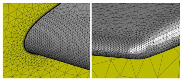
A mesh, such as this one, is considered relatively coarse to capture shocks. Therefore, this tutorial will demonstrate how a sequence of airflow mesh adaptation cycles improves the level of precision of CFD results by capturing not only the lambda shock, but also the wake and wing tip vortex produced by the ONERA M6.
