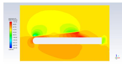
Figure 31.34: Pressure Distribution with Collective and Cyclic Trimming; Y=0 Cutting Plane
